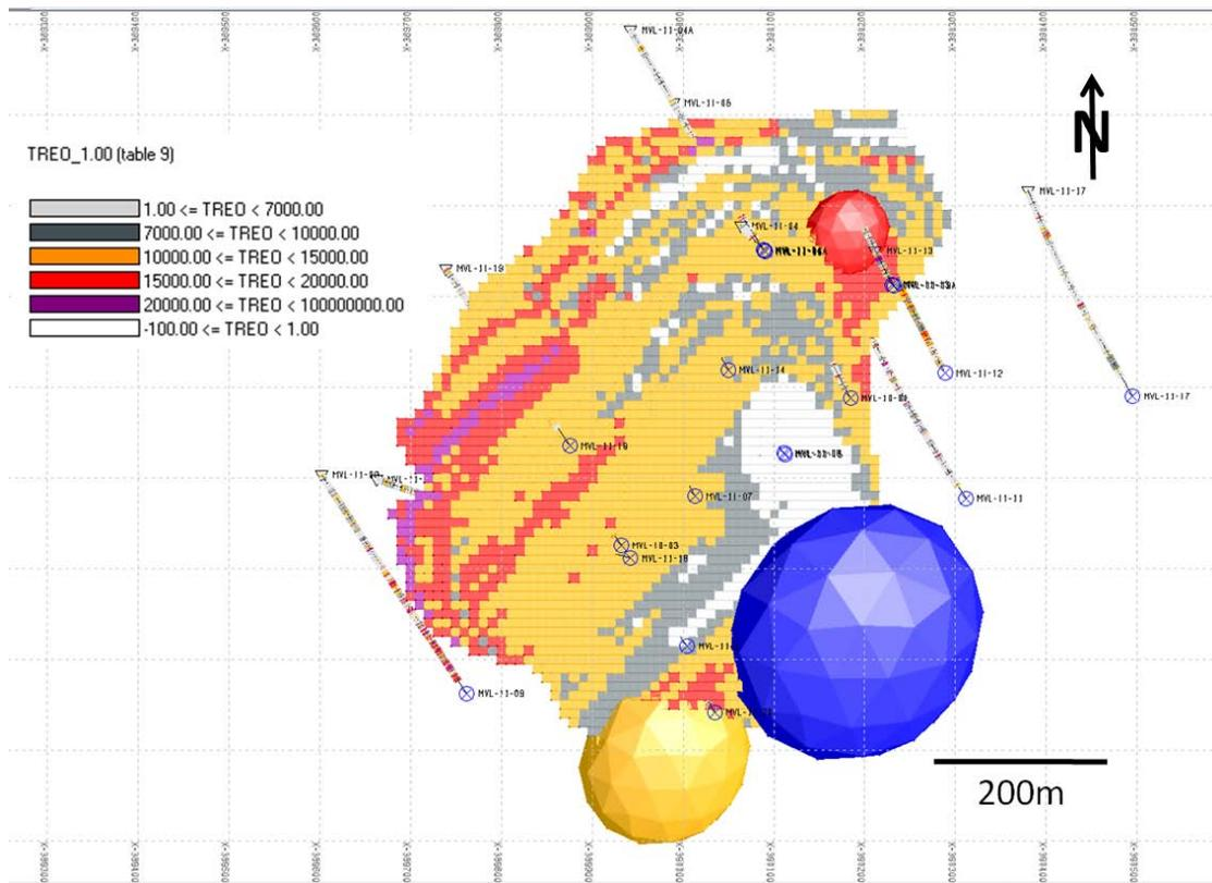
Figure 30. Plan view of the block model showing the three search ellipses. Red: first pass; Orange: second pass; Blue: third pass.
