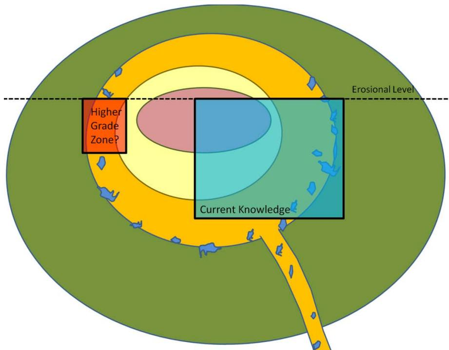
Figure 38. Conceptual model illustrating potential opportunities (red box) that may exist locally that should be tested at this early stage of exploration. The blue box represents the extent of current drilling and corresponds roughly with the area covered in the map within Figure 36. See Figure 14 for details on the lithological model.
