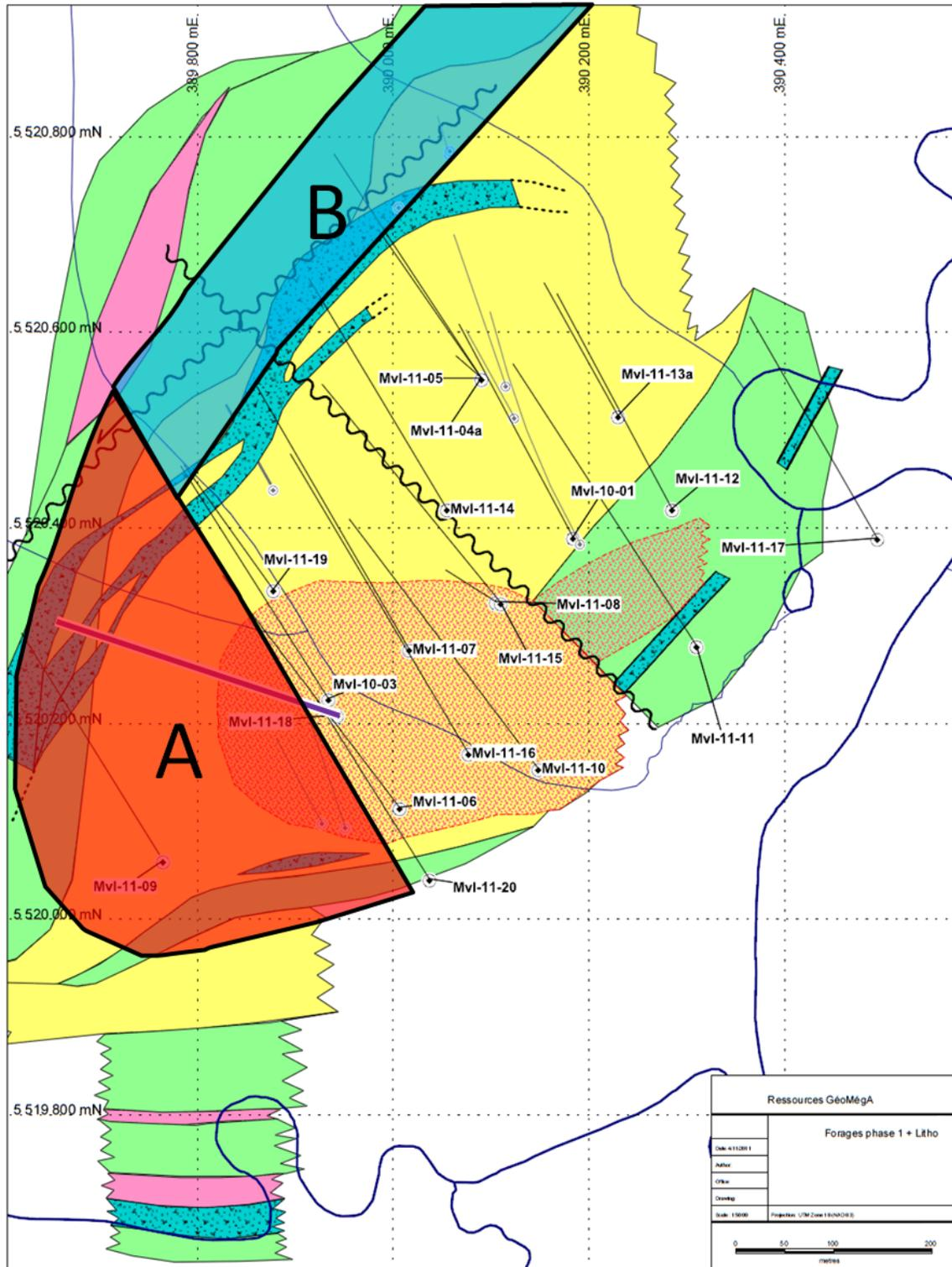
Figure 36. Geological map showing areas where SGS Geostat recommends follow-up drilling. A: High-grade zone in the S-W. B: Potential continuity of deep high grade across the Polygenetic Breccia. Yellow: Inter-layered Calciocarbonatite and Ferrocyanatite; Green: Silicocarbonatite; Pink: Calciocarbonatite; Teal: Polygenetic Breccia; Red-Stippled: Phosphate rich Carbonatite.
