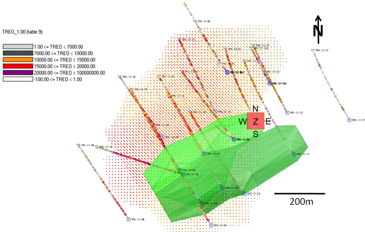
Figure 27. Plan map showing the position of the phosphate-enriched zone in green. This zone outcrops at surface and is variably enriched in REE.
