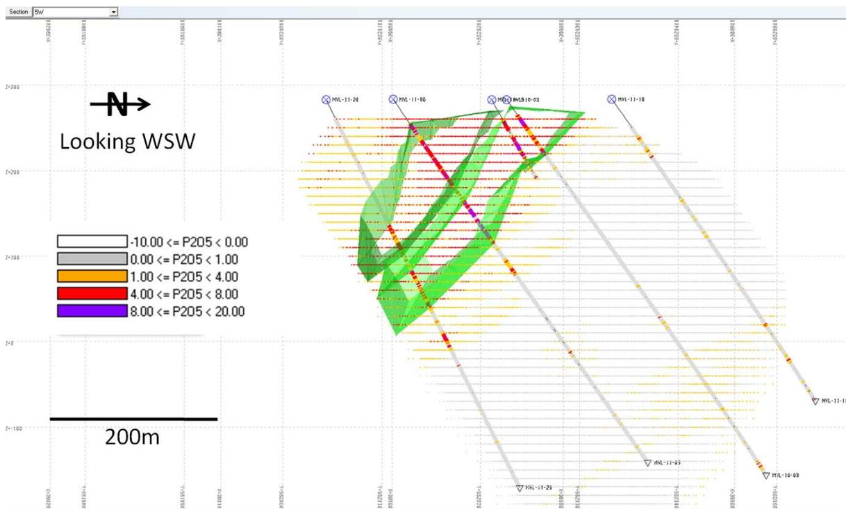
Figure 28. Section 5W showing the  $P_2O_5$  distribution. The green wireframes were drawn to outline the phosphate-enriched zone. Only a portion of the phosphate zones shown here was retained in the resource statement due to a TRED based cut-off.
