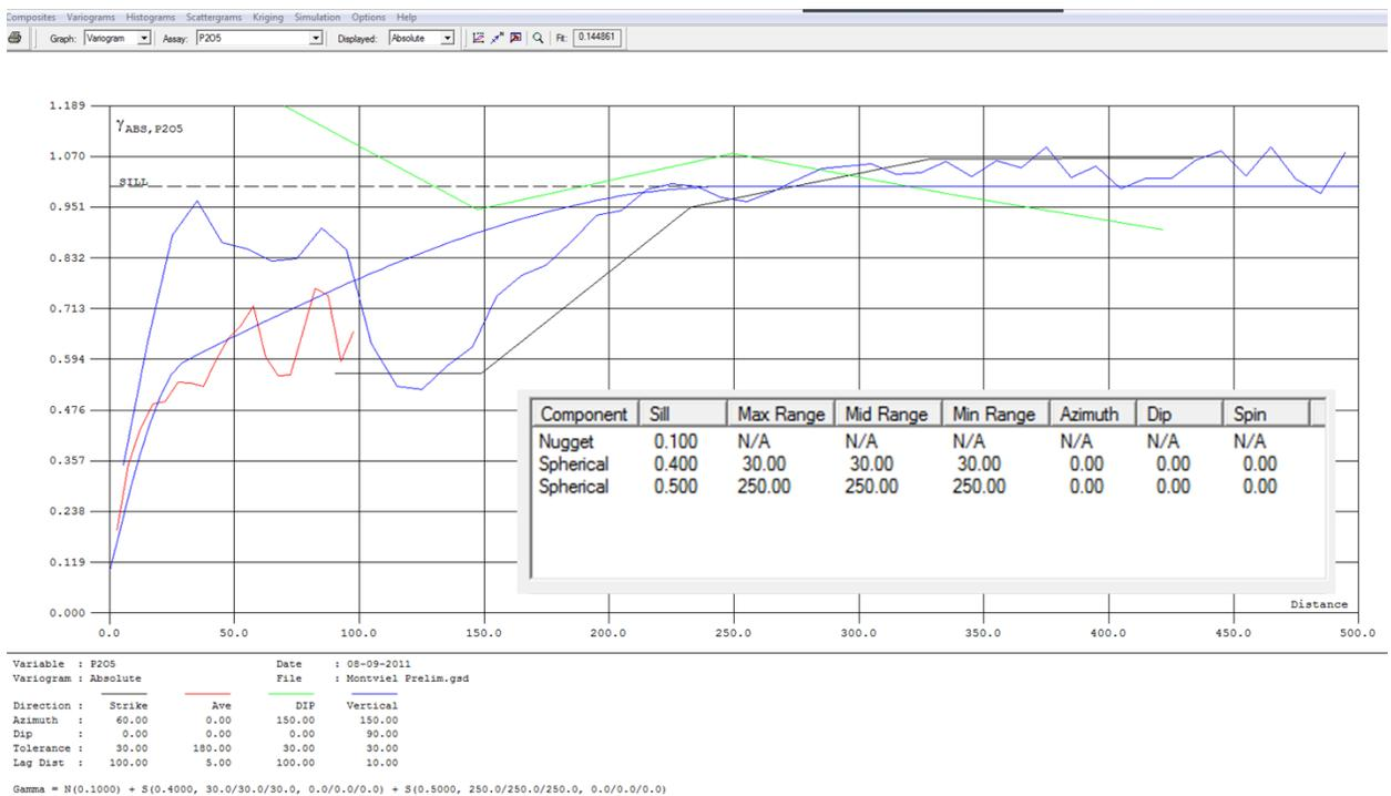
Figure 33. Variogram for P<sub>2</sub>O<sub>5</sub>. Inset is the parameters used in for the kriging based on the variance model.
