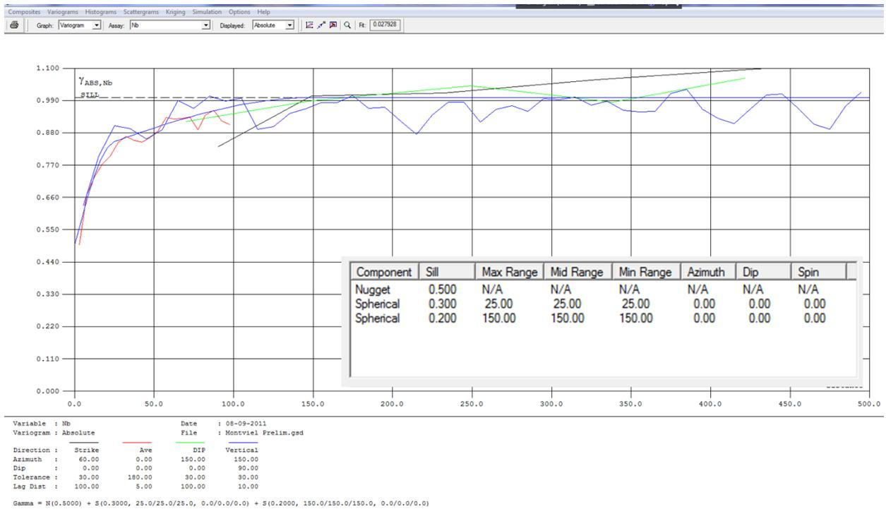
Figure 32. Variogram for Nb. Inset is the parameters used in for the kriging based on the variance model.
