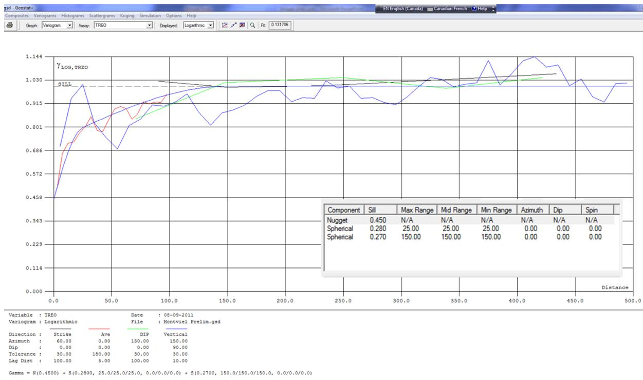
Figure 31. Variogram for TREO. Inset is the parameters used in for the kriging based on the variance model.
