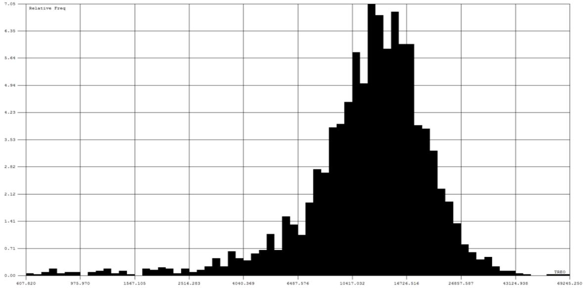
Figure 29. Histogram of TREO from composites within the mineralized envelope.
