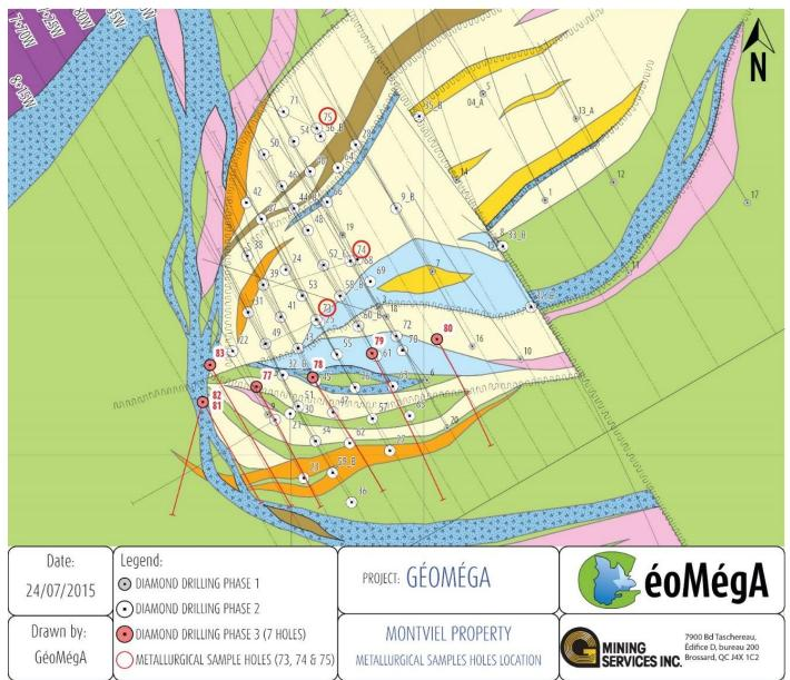
Figure 13.1: Location of the Drill Hole Used to Generate the Met Testing Composite 4
