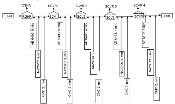
Figure 13.2: Retained REE-Nb Bulk Flotation Scheme
