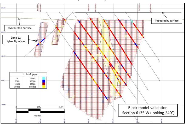
Figure 14.12: Drilling Section 6+35W Showing Block Grade vs. Composite Grade (TREO Grade)
