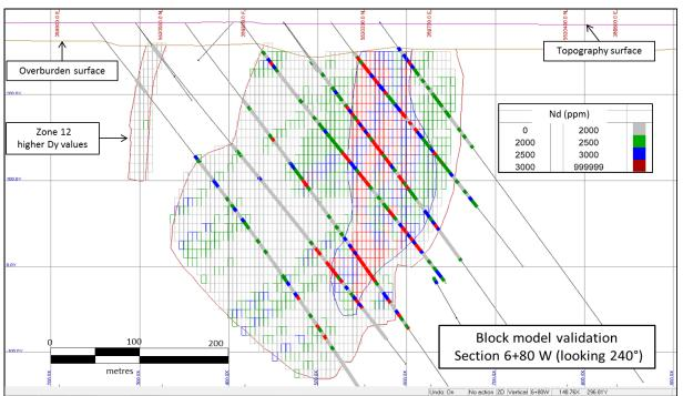
Figure 14.13: Drilling Section 6+80W Showing Block Grade vs. Composite Grade (Neodymium Grade)
