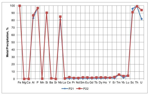
Figure 13.5: Metal Precipitations for Bulk Leach Liquor Purification
