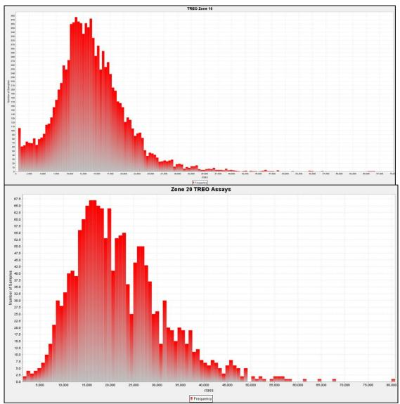
Figure 14.9: Histogram Zone 10 (lower grade) and 20 (higher grade) for TREO (ppm)
